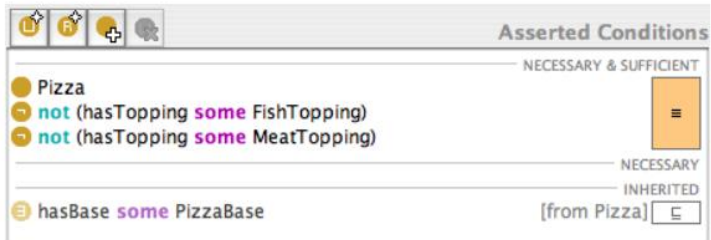
Fig. 4. An example of the Manchester OWL Syntax being used to represent the concept of a VegetarianPizza in Protégé-OWL
